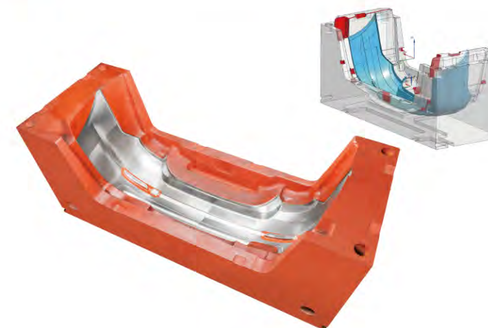
Bumper Mold Size: L900 x W2,300 xH930mm Material: FC300
